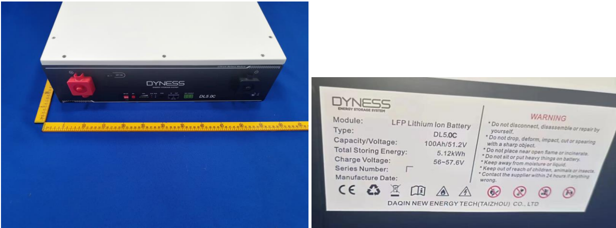
铭牌和丝印差异 (Label and Screen printing difference)
